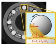
Friction on the bearing's ball surface
