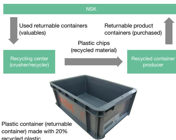
Plastic container (returnable container) made with 20% recycled plastic
