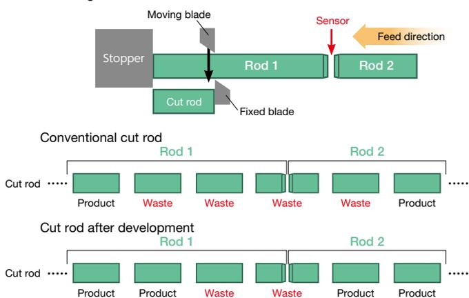
Note: Steel rods are fed continuously into a cutter and cut into fixed lengths. Lengths that are not the right size appear around the boundary between rods and cannot be used for products. In the past, four pieces including the boundary area could not be used for products, but we reduced this to two by improving the detection accuracy of the sensor. As a result, the length of rod needed to make the same amount of product was reduced by 0.7% to 1.6%.
