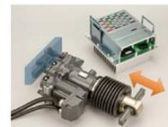
NSK vibration control actuator for train cars
