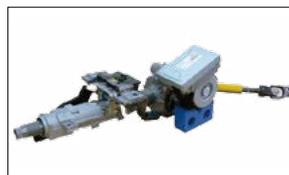
Column Type Electric Power Steering
