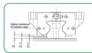
Highly dustproof V1 bottom seal is installed on the bottom face of the slide. Pay attention to possible interference with 'shoulder' set up on the
