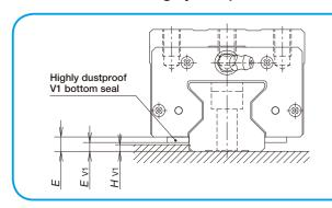
Highly dustproof V1 bottom seal is installed on the bottom face of the slide. Pay attention to possible interference with 'shoulder' set up on the machine base.
