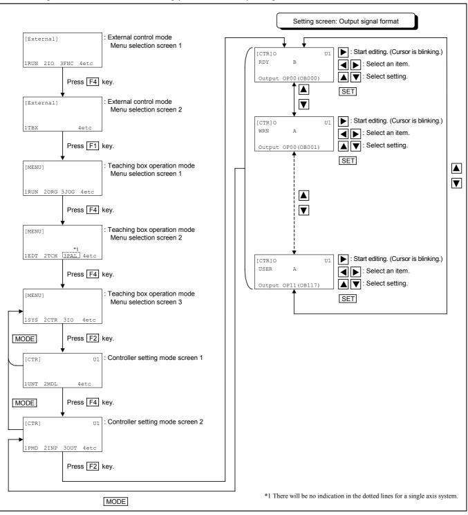
Figure 9-20: Parameter setting procedure: Output signal format
