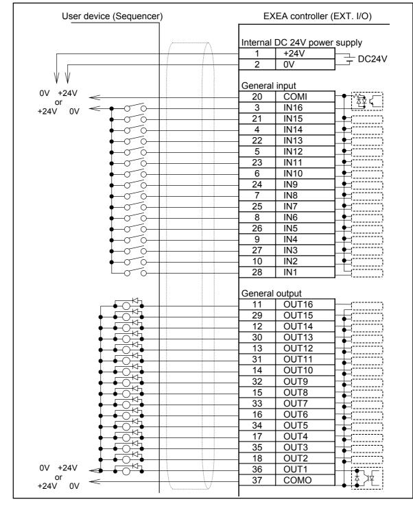
Figure 7-14: Sample wiring diagram
