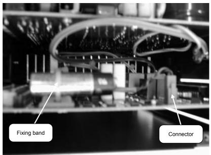
Photo 12-8: The way how the battery is fixed
