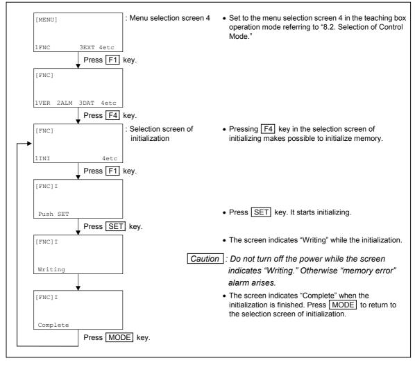
Figure 13-5: Procedure of initializing memory.
