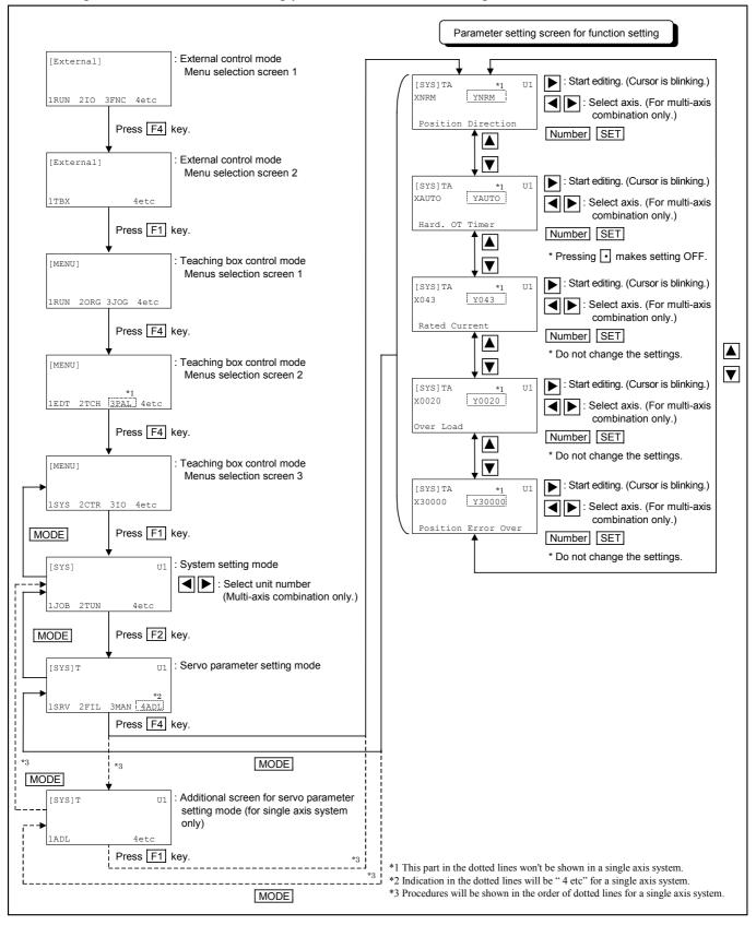
Figure 9-12: Parameter setting procedure: Function Setting
