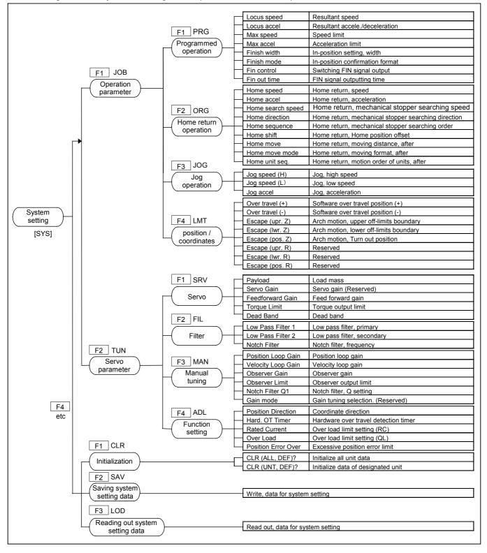
*Figure 9-2: System setting mode (Multi-axis controller)*
