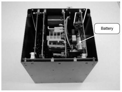
Photo 12-7: A view when the cover is removed. <Single axis controller>
