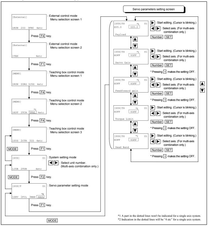
Figure 9-9: Parameter setting procedure: Servo
