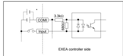
\* You may connect here as "Minus common" when the polarity of the external power supply is reversed.
