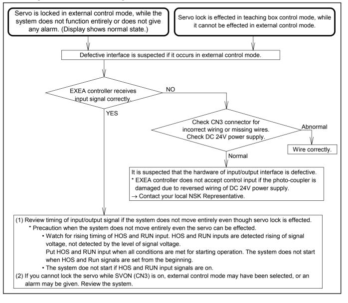
Figure 14-5: Troubleshooting when servo-lock is not effected
