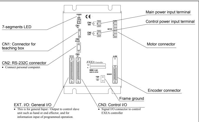
Figure 5-1 : EXEA controller (Single axis)
