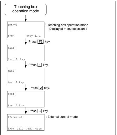
\* When this procedure is executed while the system is operating, the controller terminates the programmed operation and gets in [Eternal] control mode.
