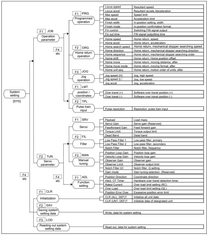
Figure 9-1: System setting mode list (Single axis controller)
