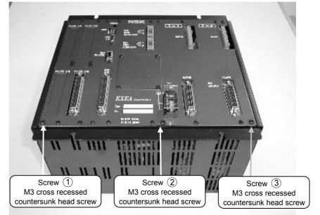
Photo 12-3: Indication of the screws to be removed. (1) <2 axes controller>
