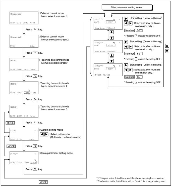
Figure 9-10: Parameter setting procedure: Filter
