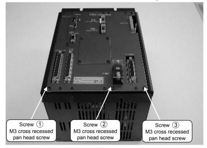
Photo 12-2: Indication of screws to be removed <Single axis controller>
