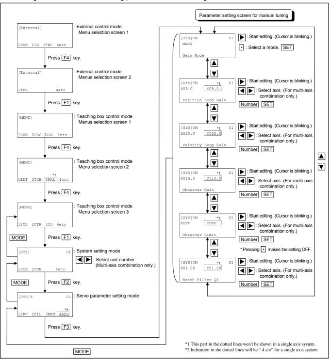
Figure 9-11: Parameter setting procedure: Manual tuning
