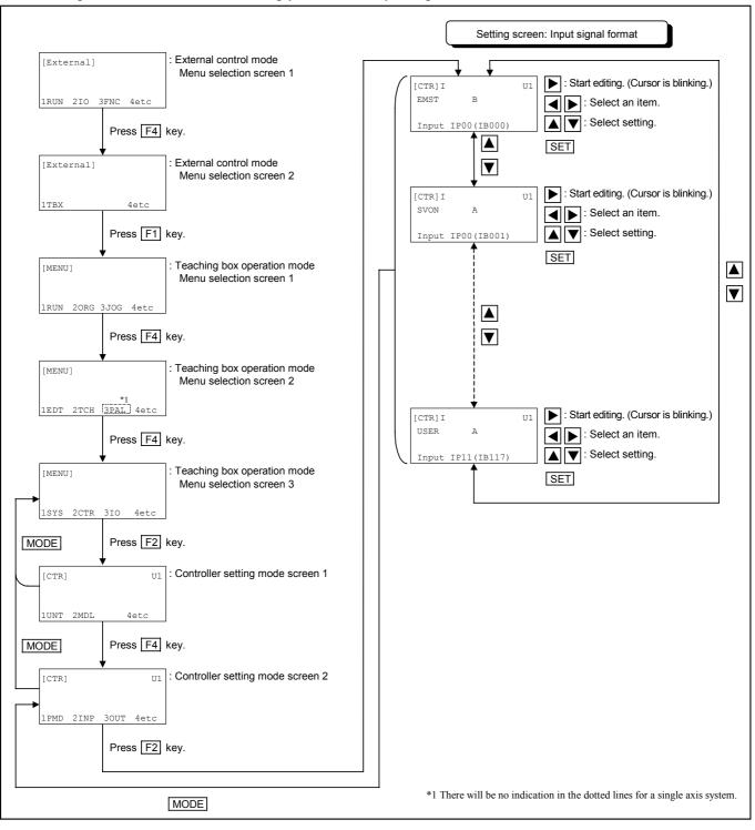
Figure 9-19: Parameter setting procedure: Input signal format
