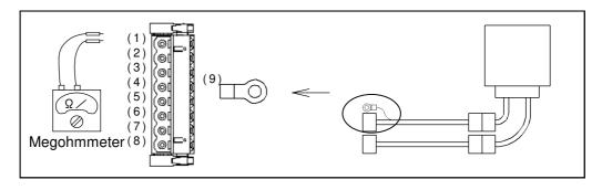
Fig A-11: Check the Motor only
