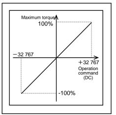
Caution • Depending on the parameter DI setting, the polarity of the DC command is reversed.
