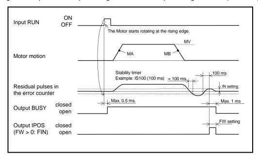
• The System always confirms completion of positioning every time inputting pulse pauses in the pulse train command operation. If the intervals of inputting pulses are intermittent, set the parameter IS longer because the outputting IPOS signal will be unstable.
