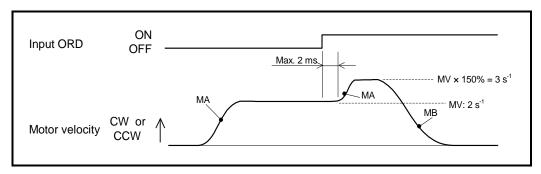
Fig 8-4: Signal timing of the ORD input: (In case of OV50)
