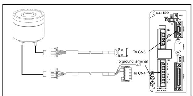
Fig 3-6: Connection of cable set
