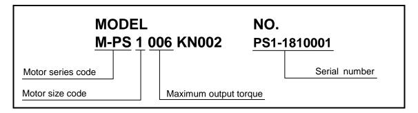
Fig 3-2: Indication on the nameplate sticker of Driver Unit
