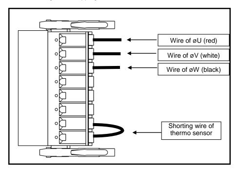
2) Remove the shorting wire of thermo sensor using a removing tool. Connect the cable of regeneration resistor and the sensor cable. A thicker cable pair is the resistor cable while a thinner cable pair is the sensor cable. No polarity is set to the both pairs.
