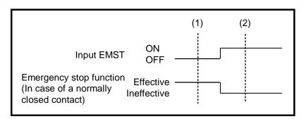
♦ The "Table A-2: Read out of the monitors IO0 and IO1 when the input EMST is a normally closed contact" below shows the comparison of the readouts of the monitor IO0 and IO1 at the moment of (1) and (2) in "Fig A-3: Port polarity and ON/OFF of the input EMST" above.
