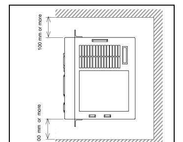
Fig 3-5: Installation of Driver Unit
