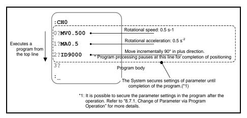
♦ The channel number 0 is used for the program. Input the command SP0.(Fig 6-7: Program example)
