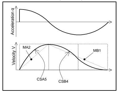
1) Specify an acceleration profile. For example, set the half sine profile for acceleration and the cycloid pattern for deceleration.
