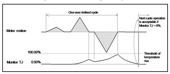
Fig 7-33: Check of thermal loading after one cycle
