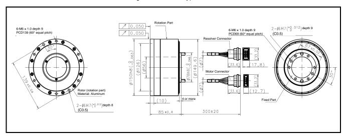
Fig 2-20: PS3030 type Motor
