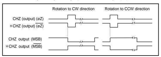
Provided the control of the phase Z is used to specify the position scale of the Motor, be sure to use the rising edge of the signal.
