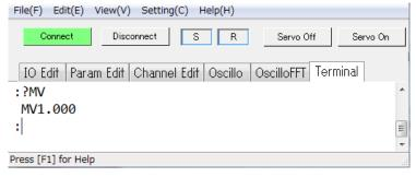
2) Set the parameter MV to 0.5 [s<sup>-1</sup>] Enter as **Parameter code** + **data**
