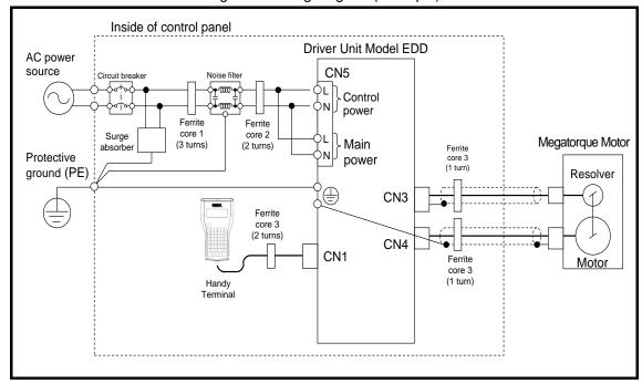
Figure 1: Wiring diagram (Example)
