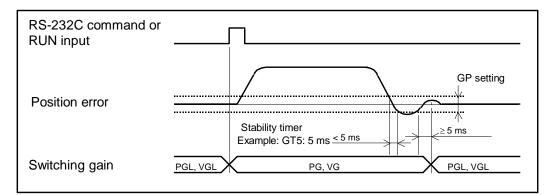
Fig 8-13: Functioning timing of gain switching
