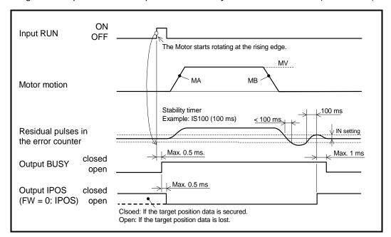
• In the pulse train command operation, the System always confirms completion of positioning every time inputting pulse pauses. If the intervals of inputting pulses are intermittent, set the parameter IS longer because the outputting IPOS signal will be unstable.
