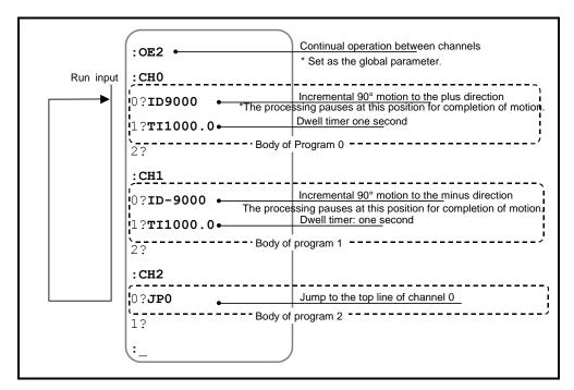
• Specify the channel 0 by the input PRG, then input the RUN signal to alternate the incremental positioning of 90° to the plus direction and the minus direction having one second dwell time between.
