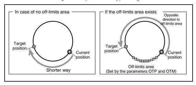
• The function of shorter way positioning is available for the absolute positioning commands shown in the table below.
