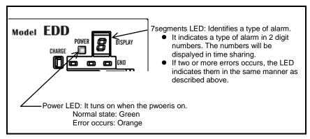
Fig 3-11: In normal state
