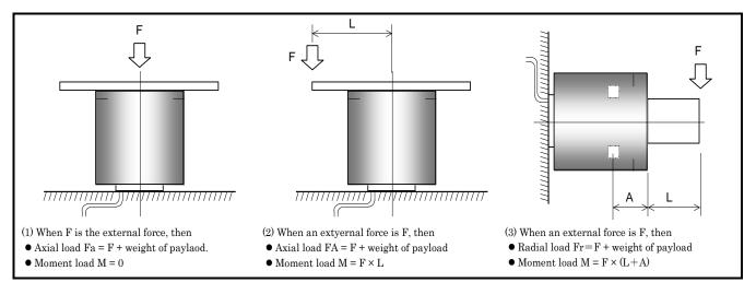
Table 2-9: Dimension A (Distance between the bearing and the rotor surface)
