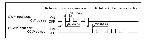
Fig 6-19: When the parameter is set to PC1 (Pulse and direction format, PM2)
