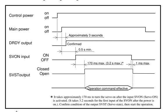
Fig 3-14: Signal timing for Power on and Servo on
