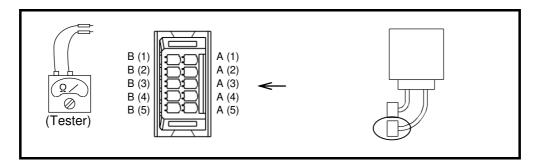
Table A-7: Checking points of a resolver with absolute position sensor and winding resistance
