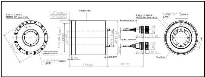
△ Caution: The bend radius of the motor cable lead (Ø 7) and the resolver cable lead (Ø 7) should be R30 [mm] or more.
