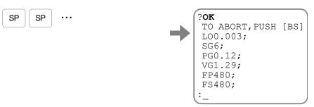
• For the EDD MEGATERM terminal screen display, the parameters set by automatic tuning are displayed in batch.
