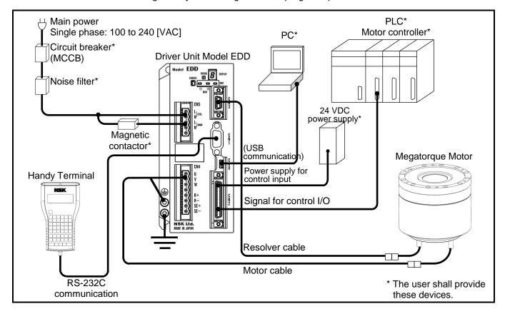
Fig 2-2: System configuration for pulse train operation and analog input operation
