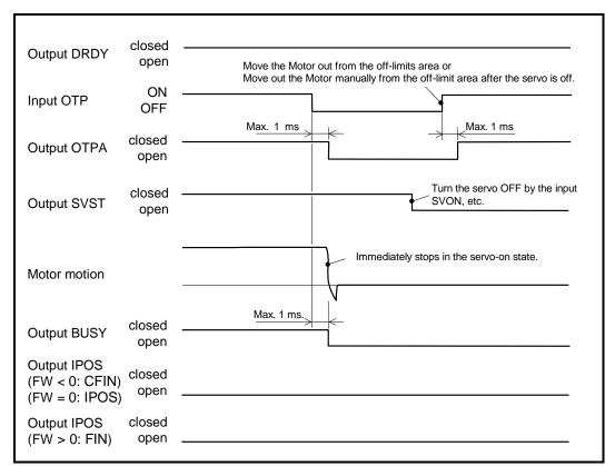
Fig 7-10: Signal timing of the input OTP and the output OTPA (negative logic)
