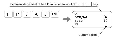
Caution: An input of the keys SHIFT + will alter the increment or the decrement of an input of the (+) and (–) keys to 10 times of the current setting.
