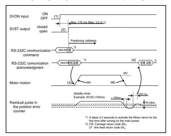
Fig 6-23: Signal timing of an RS-232C communication positioning
