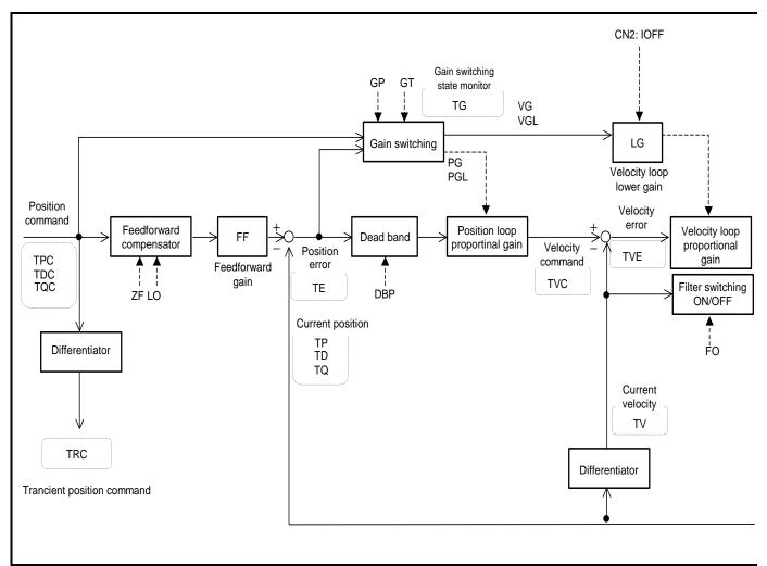
Fig 8-11: Servo block diagram
