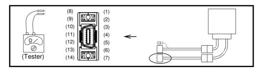
Fig A-8: Check the Motor only
