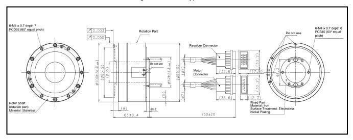
Fig 2-16: PS1006 type Motor
