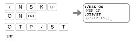
The parameter OTP is set by teaching. Input the SP key to put the prompt ": (colon)" on the bottom line.
