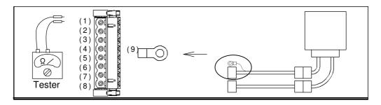
Fig A-6: Check the Motor only
