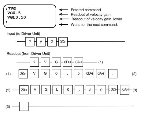
Caution: When the parameter MM is set to MM1, the prompt semicolon (:) is added to the end of line. Input of  $[20_H]$  is required every time the prompt (;) appears.
