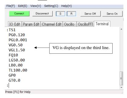
All the parameters belonging to TS1 and the prompt ":" (colon) will appear on the screen to indicate the completion of readout.
