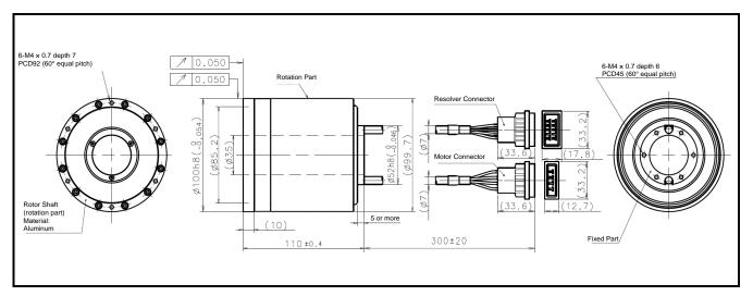
Fig 2-18: PS1018 type Motor
