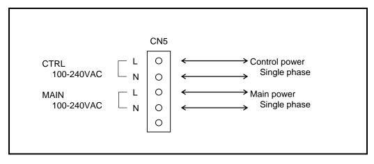
Danger: Do not connect or disconnect the connector when the cable is energized.
