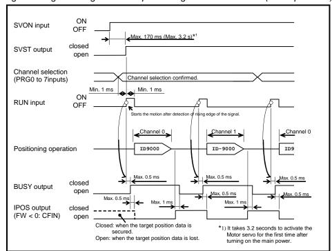
Sequence code: Continual positioning between channels (without the input RUN)
