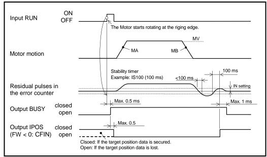
• The System always confirms completion of positioning every time the inputting pulses pause in the pulse train command operation. If the inputting pulses are intermittent, set the parameter IS longer. Otherwise the output IPOS signal will be unstable.
