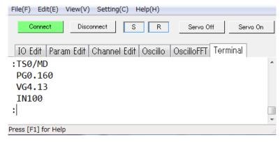
The parameters whose setting has been altered from the shipping set are identified. The prompt ":" (colon) will appear on the screen to indicate the completion of readout.
