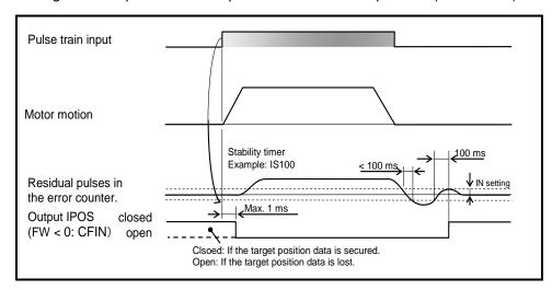
• The parameter FW sets the minimum holding time to keep the output IPOS open for the confirmation even for a very short operating time. (The unit is 1 millisecond. When the parameter is set to FW10, the time is 10 ms.)
