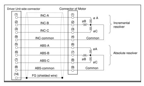
Insulation resistance check of Motor winding
