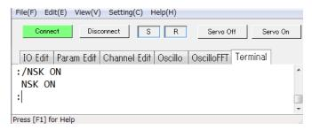
The acknowledgment appears on the screen, and the colon appears indicating the normal standby state for command entry. Then set a parameter or a command.
