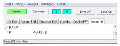
The current position is read out continuously. An input of the BS key will resume the readout and the prompt changes to ":" (colon).
