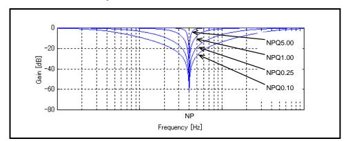
Fig 8-12: Characteristics of notch filter
