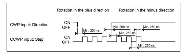
Fig 6-20: When the parameter is set to PC4 (øA/øB format, PM2)
