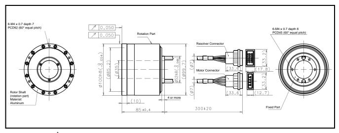
Caution: The bend radius of the motor cable lead ( $\phi$ 7) and the resolver cable lead ( $\phi$ 7) should be R30 [mm] or more.
