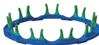
The new cage is lighter, stronger, and more rigid to control deformation and avoid contact with the outer ring
