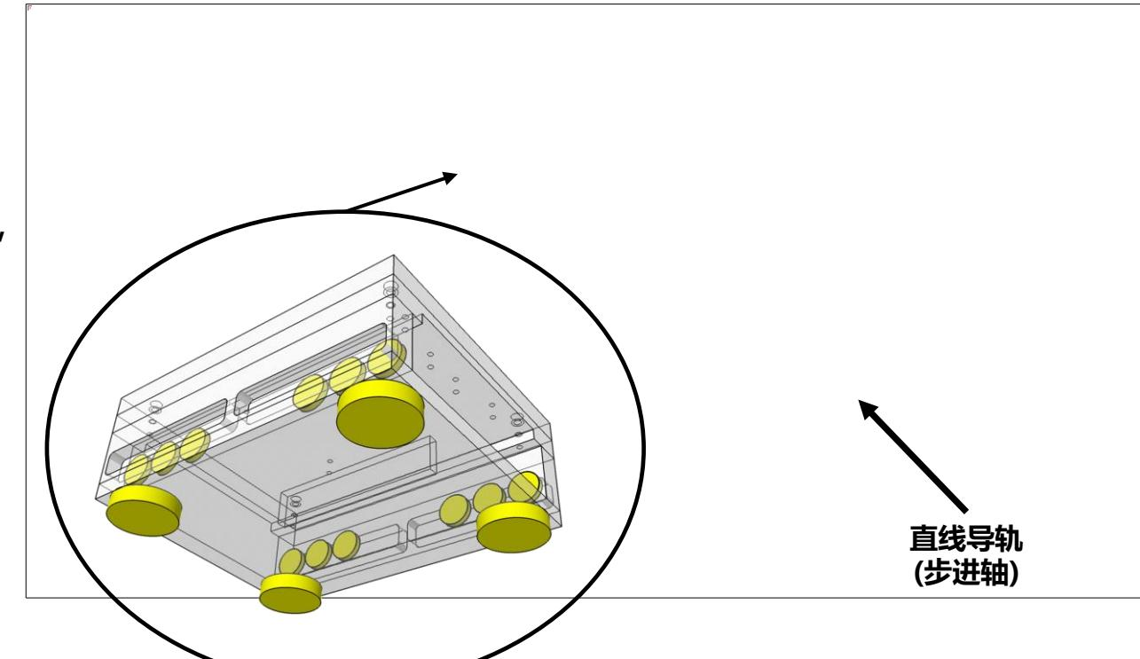
Combining a high-precision air slide and linear guide
