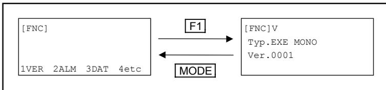
Figure 13-8: Screen indicating software version number. (Example of two axes combination)
