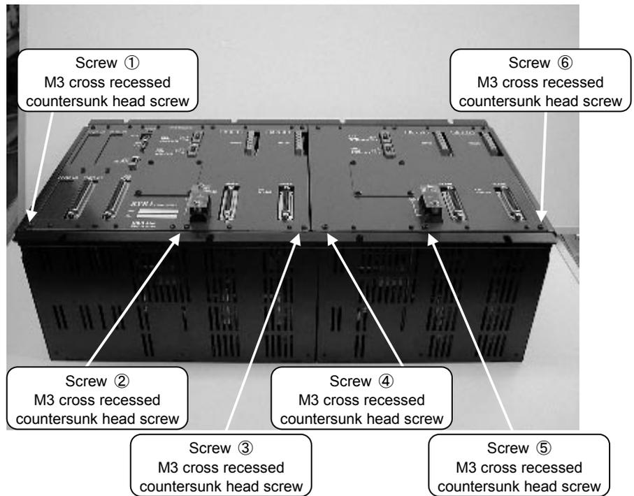
Photo 12-6: Indication of screws to be removed (2)
