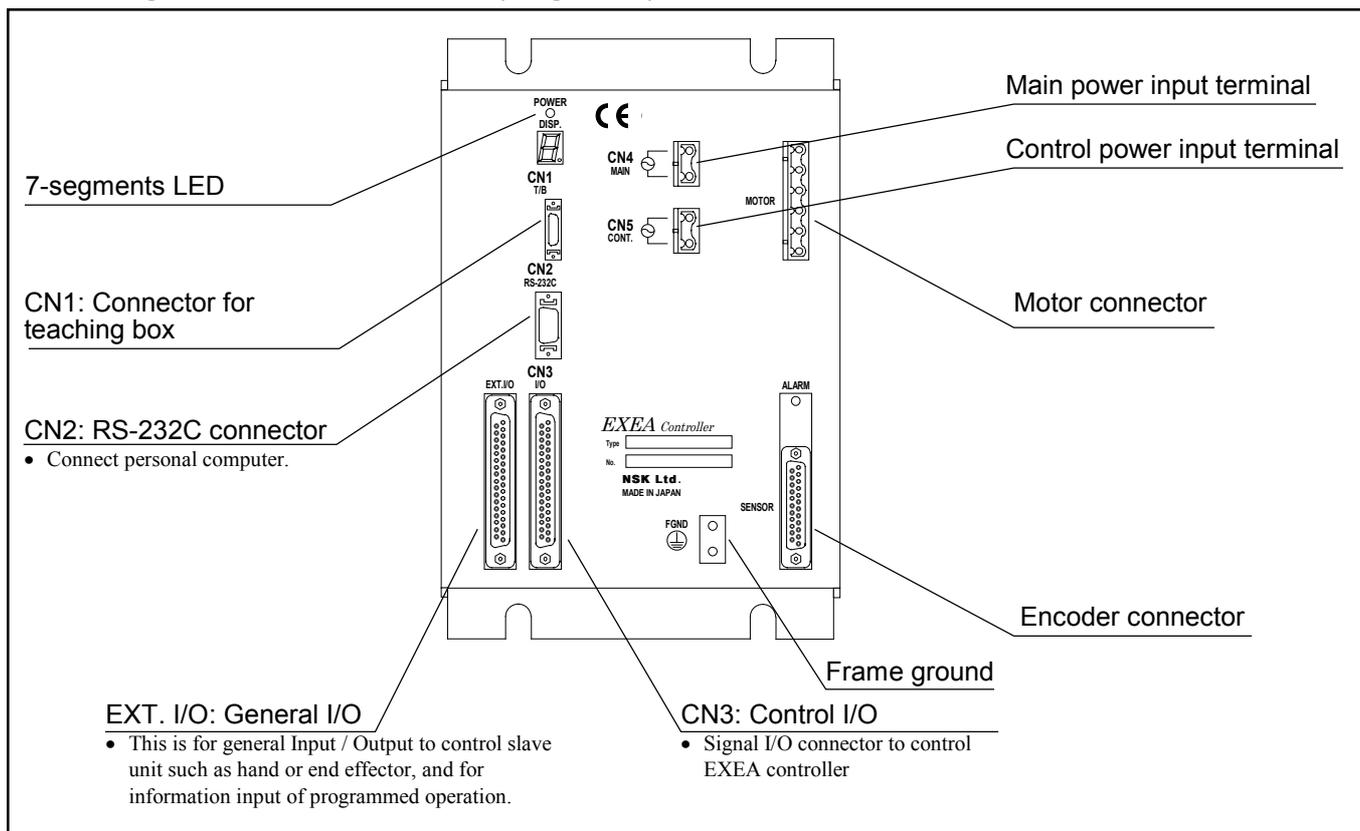
Figure 5-2 : EXEA controller (2 axes)
