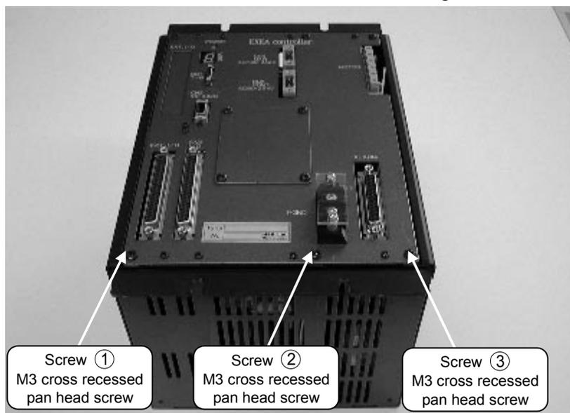
Photo 12-2: Indication of screws to be removed <Single axis controller>
