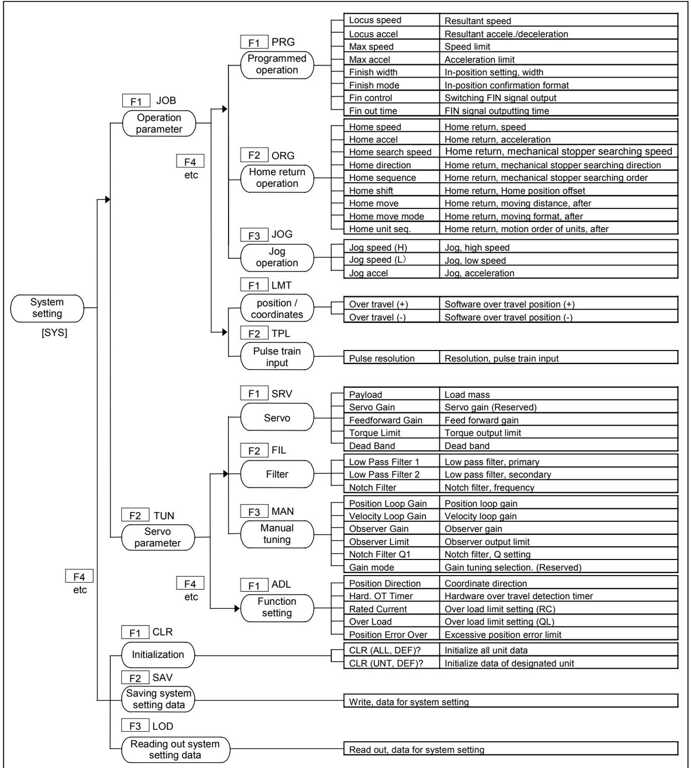
Figure 9-2: System setting mode (Multi-axis controller)
