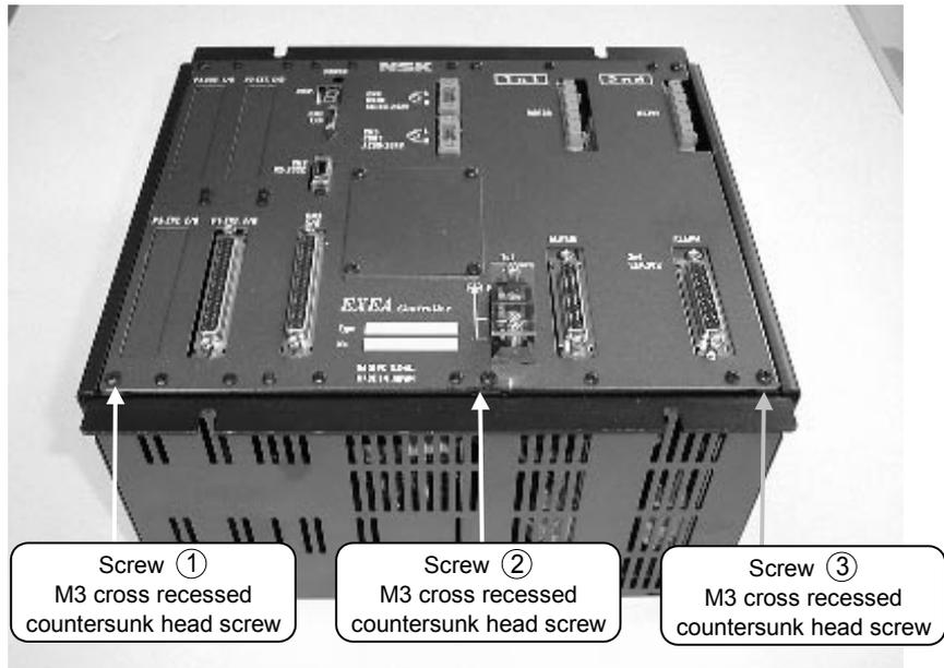
Photo 12-4: Indication of the screws to be removed (2) <2 axes controller>
