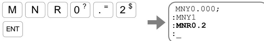
Fig 7-35: How to customize an analog monitor
