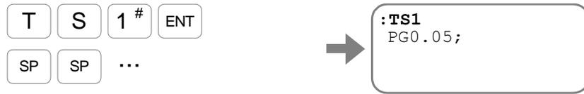
Firstly the parameter PG (Position gain) is read out. Then each input of `SP` key scrolls to following parameters that belong to the group TS1. Record the parameter values for future reference.
