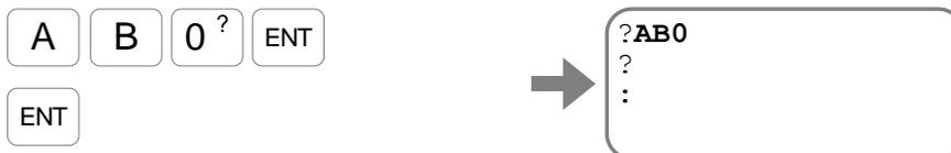
Thus the input EMST (Emergency stop) has been changed to the normally open contact.
