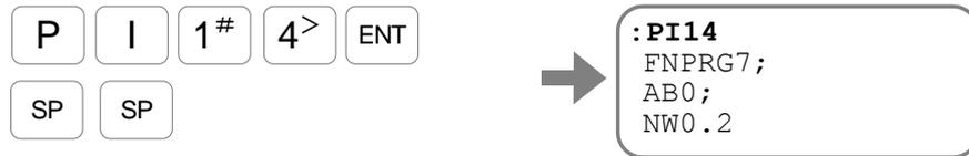
Every input of the **SP** key reads out the parameter AB and the parameter NW.
