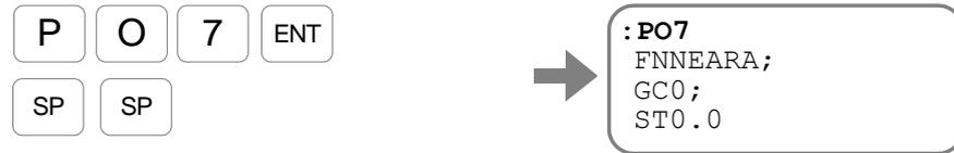
Every input of the  key displays the parameters GC and ST respectively.
