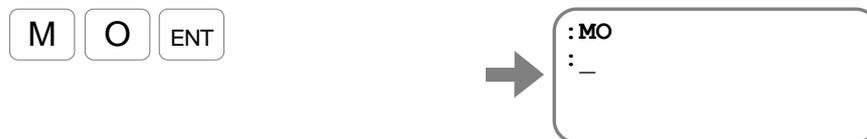
This will prohibit the Driver Unit from activating the Motor servo even the main power is turned on and the input SVON (Servo on) is activated.
