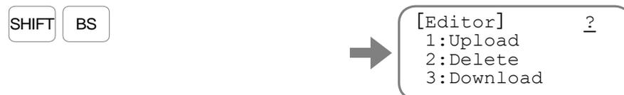
(2) Execute downloading (Transfer the setting to the memory of the Driver Unit from the Handy Terminal). Press the keys in order of **[3]** and **[ENT]** to change the display menu for inputting the file number.
