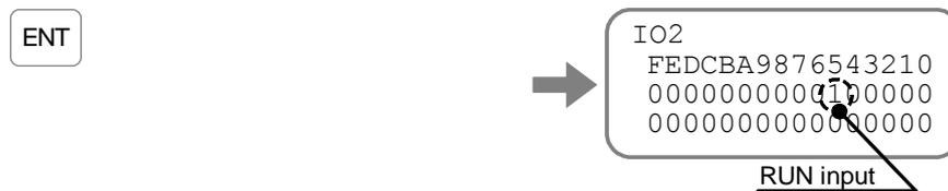
The first line below the guide **5** represents the readout of the input RUN.
