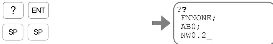
Every input of the **[SP]** key displays the parameters FN, AB and NW.
