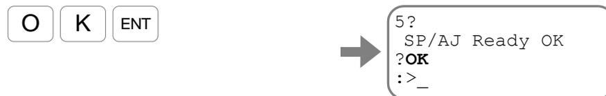
The Motor starts a cyclic motion as soon as you input the OK message. (Firstly, the Motor moves in CW direction.)
