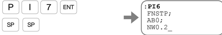
Every input of the **[SP]** key displays the parameters AB (Input port polarity) and NW (Anti-chattering stability timer).
