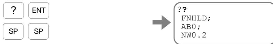
Every input of the **SP** key reads out the parameter FN setting, the parameter AB, and the parameter NW.
