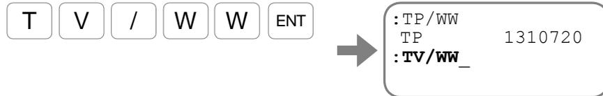
Thus, two conditions can be monitored simultaneously. You may input the command in this state.
