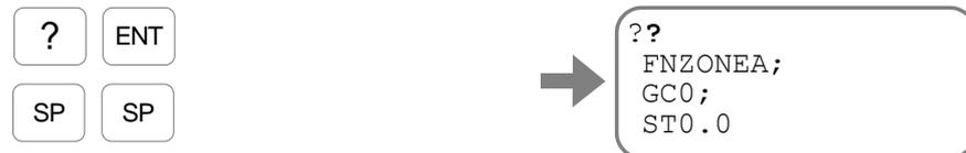
Every input of the  key displays the parameter FN and GC respectively.
