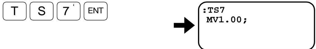
The screen will show firstly the setting of the parameter MV for the velocity of the Motor.
