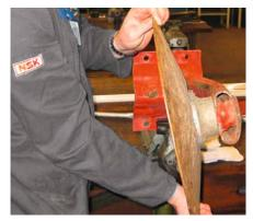
An NSK employee removing the unit from the machine arm.
