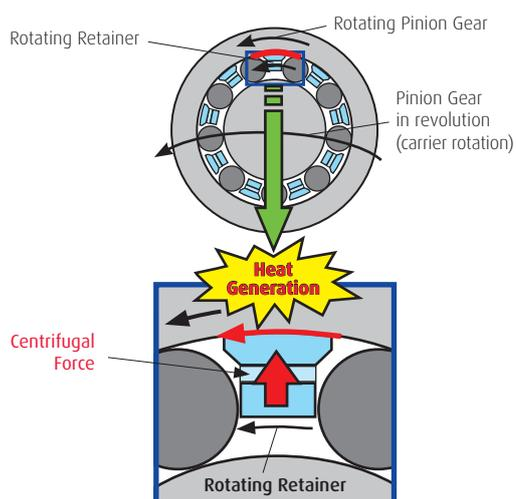
Higher-speed design of planetary
