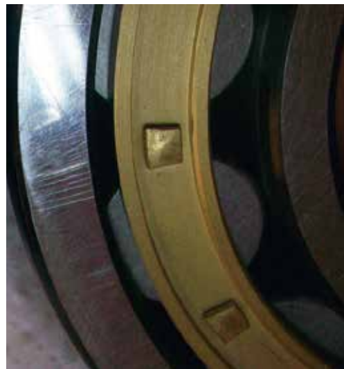
B. Counterfeit Bearing
