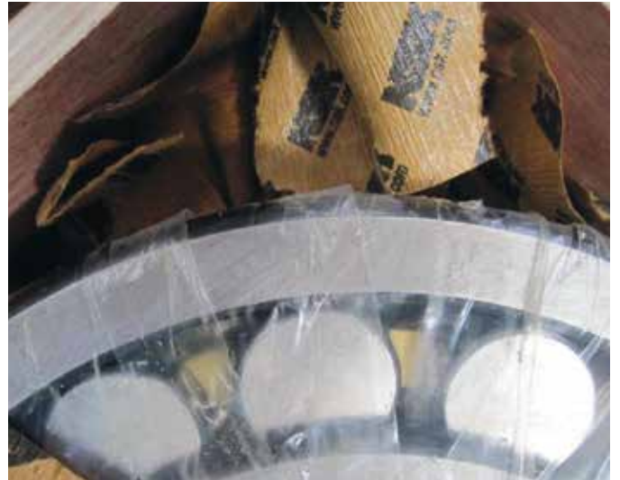
B. Counterfeit Bearing
