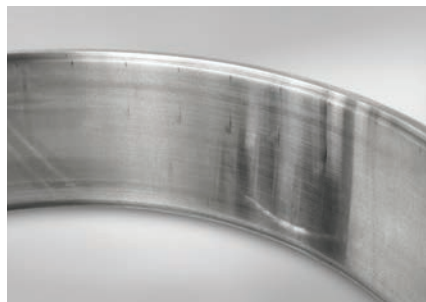
Part: Outer ring of a double-row cylindrical roller bearing Observation: Axial scratches at roller pitch intervals on raceway surface Cause: Inclination of inner and outer rings during mounting
