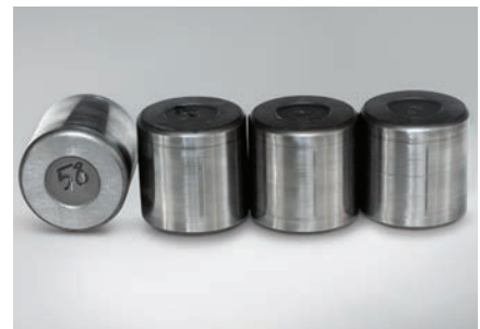
Part: Rollers of a cylindrical roller bearing Observation: Axial scratches on rolling surface Cause: Inclination of inner and outer rings during mounting
