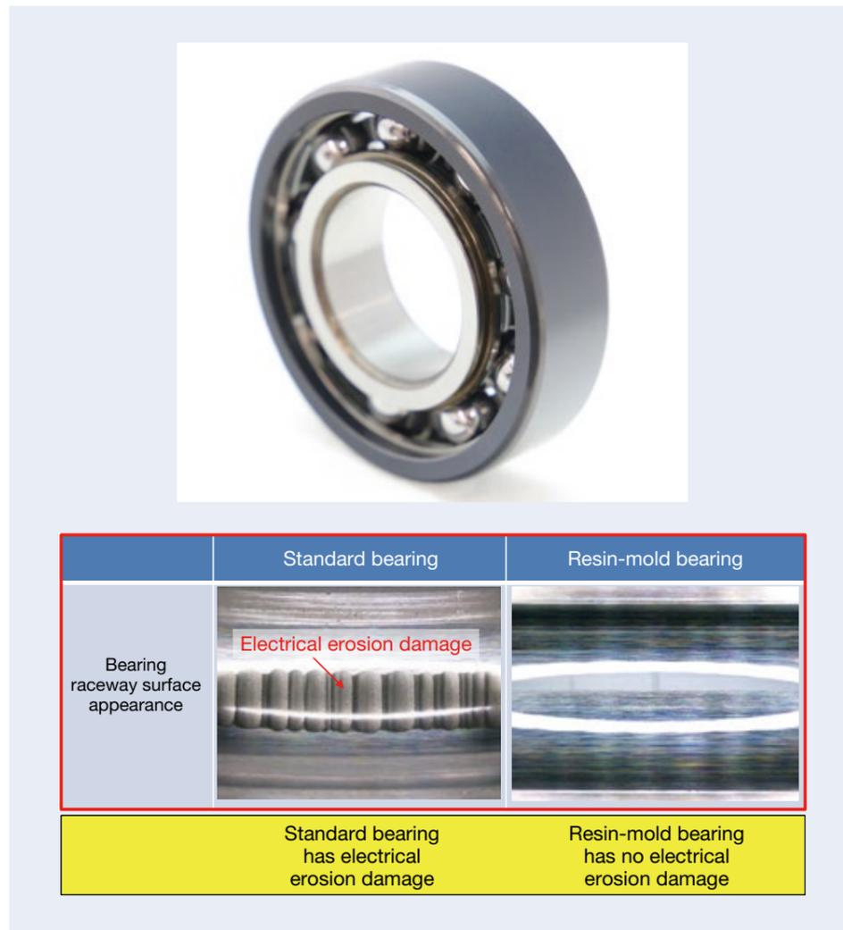
Photo 3 Resin-mold insulated bearing and electrical erosion test results
