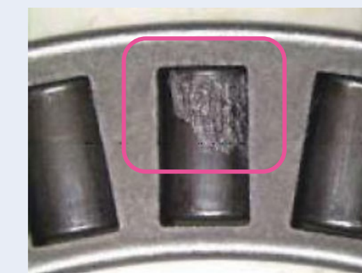
Fig. 5 Edge load spalling of thrust needle roller bearing under a tilted environment
