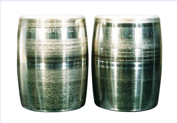
Fig. 7 Smearing damage (rolling surface of rollers)
