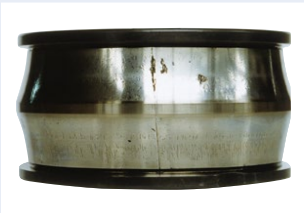
Fig. 6 Inner ring fracture (spherical roller bearings)
