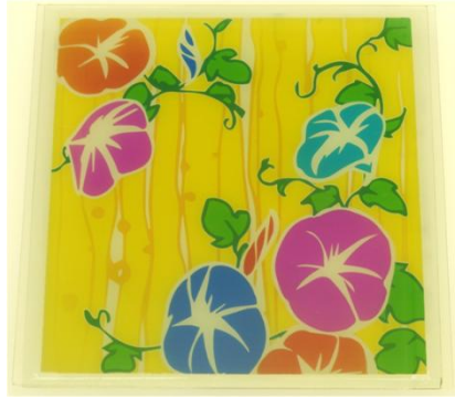
Fig.10 Dye-sensitized solar cell panel fabricated by inkjet printing
