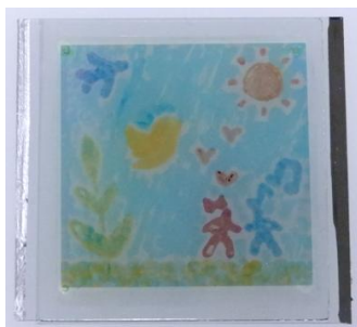
Fig.8 Dye-sensitized solar cell fabricated using titanium oxide dyed with dye pens
