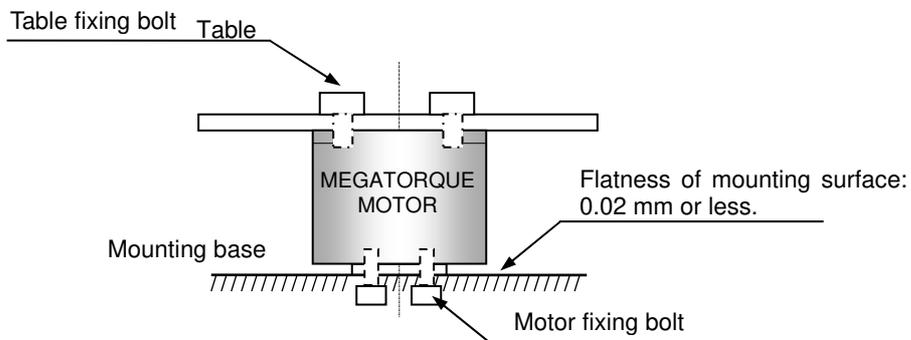
Since the installation condition shown below can cause mechanical resonant vibration or failure of estimation of magnetic pole due to low rigidity of the mounting base and the load, installation of motor to mounting base and load to motor have to be secure and rigid.
