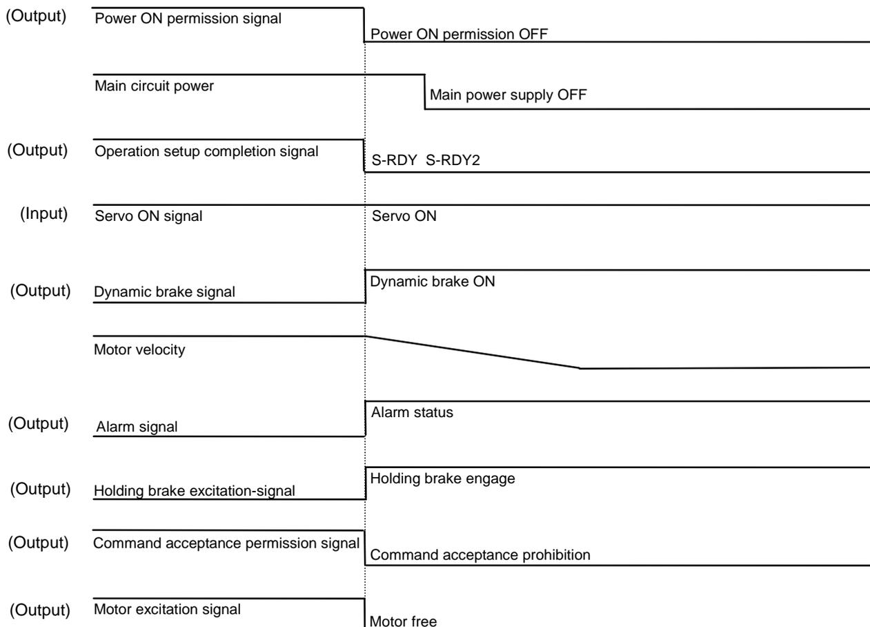
Stop by servo brake at alarm
