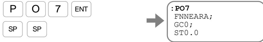
Every input of the **[SP]** key displays the parameters GC and ST respectively.
