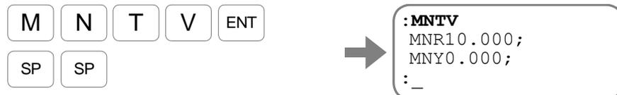
The screen indicates the default. The monitor center is set to  $0 \text{ [s}^{-1}\text{]}$  (MNY0.000) and the output range is set to  $\pm 10 \text{ [s}^{-1}\text{]}$  (MNR10 000). Input the **[SP]** for the prompt “: (colon)”.
