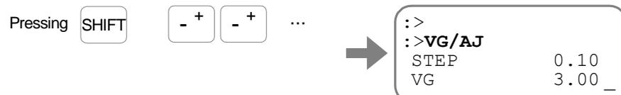
Observe how the motion of the Motor gets crisper as the setting of VG gets higher.
