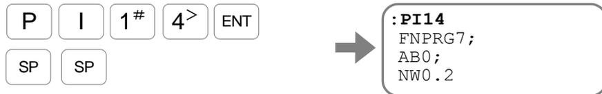
Every input of the **[SP]** key reads out the parameter AB and the parameter NW.
