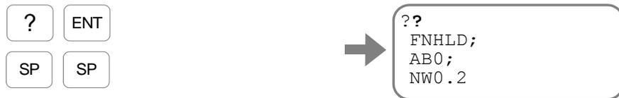
Every input of the **[SP]** key reads out the parameter FN setting, the parameter AB, and the parameter NW.
