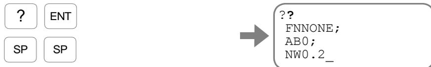
Every input of the **[SP]** key displays the parameters FN, AB and NW.
