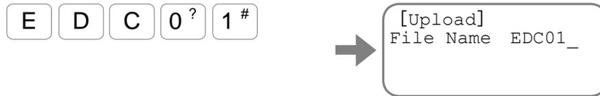
An input of the **[ENT]** key calls up the confirmation screen to start uploading.
