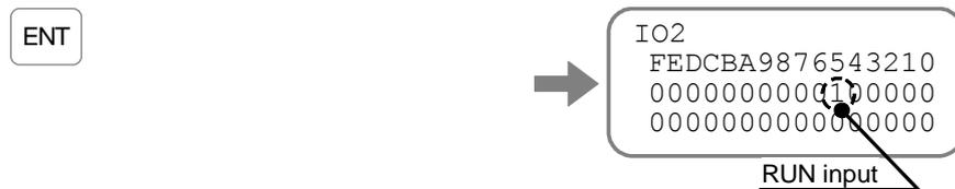
The first line below the guide 5 represents the readout of the input RUN. The readout is applied the parameter AB (Input port polarity), and thus the readout will be 1 if the input RUN is effective.
