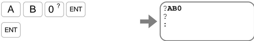
Thus the input EMST (Emergency stop) has been changed to the normally open contact.
