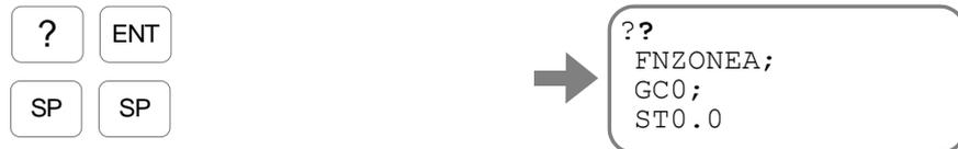
Every input of the **[SP]** key displays the parameter FN and GC respectively.
