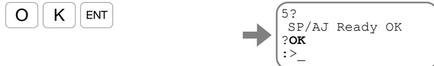
The Motor starts a cyclic motion as soon as you input the OK message. (Firstly, the Motor moves in CW direction.)
