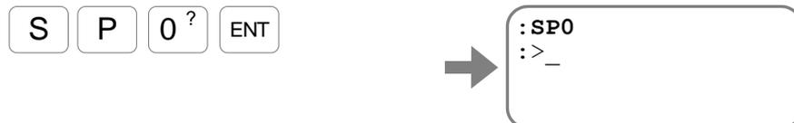
The Motor moves 90° in the plus direction. The prompt is changed to “:>” from the colon.
