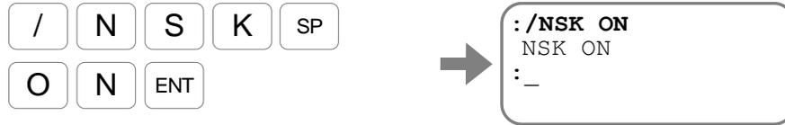
The acknowledgment appears on the screen, and the colon appears indicating the normal stand-by state for command entry. Then set a parameter or a command.
