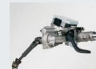
Column type electric power steering (EPS) systems
