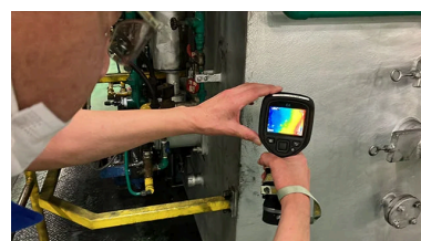
Measuring the surface temperature of a heat treatment furnace (Haruna Plant)
