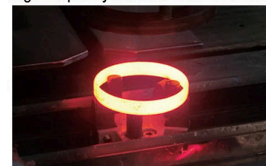
Heating the target part only
