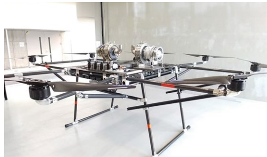
High payload emergency supply delivery drone equipped with a gas turbine generator (Photo courtesy of Aero Development Japan, Inc.)
