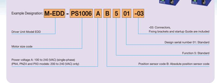
Z Series, PN Series with brake, and PN Series use the same Driver Units. Refer to Section 9 "Motor and Driver Unit Combination" for more details on applicable models
