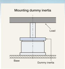
· Inertia of a dummy load shall be approximately 20% of the load inertia. When a speed reducer mechanism is used, it shall be
