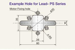
If inserting the PS Series connector through the bottom of the base, we recommend making a larger hole than that in this figure.
