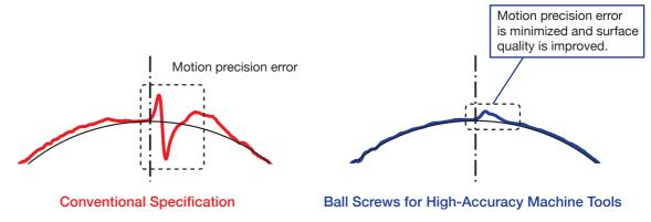
Motion precision error after servo control correction (schematic)
