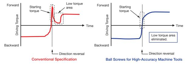
Variation of drive torque during direction reversal (schematic)
