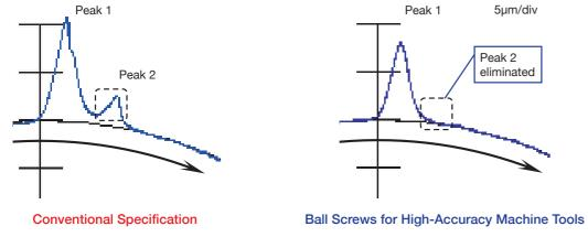
Example circularity error when reversing direction of circular interpolation
