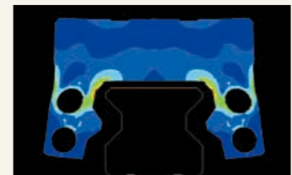
Example of roller slide deformation analysis
