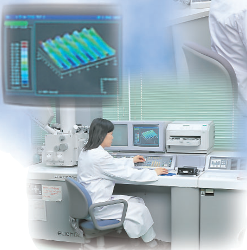
Field emission electron probe microanalyzer for surface analysis
