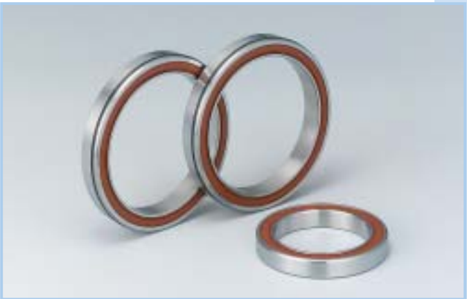
Long Life Coupling Support Bearings for 4WD Vehicles. Thin walled and large diameter bearings for 4WD coupling. These bearings with large bore and minimized outer diameter have superior heat resistance, high load capacity, and sealing performance against mud and turbid water.
