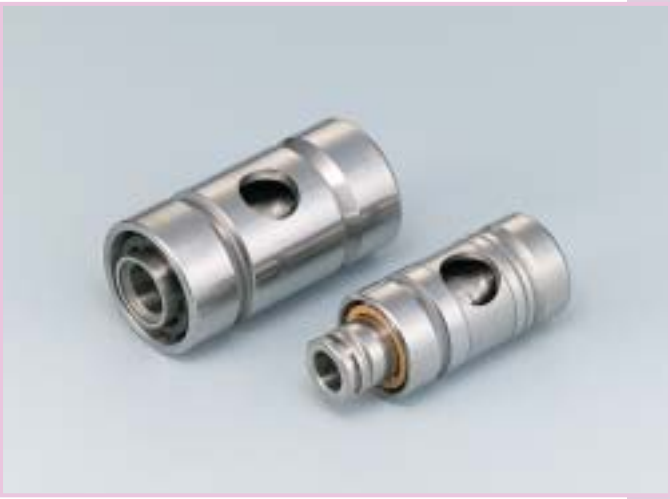
Ball Bearings for Turbocharger The cartridge bearing has little mechanical loss while requiring no preload setting.
