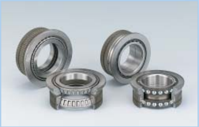
Long Life Double Row Bearings with Outer Ring Splines The outer ring has a mounting flange and splines, which attach to the one-way clutch. This affords greater compactness of FF-type automatic transmissions.
