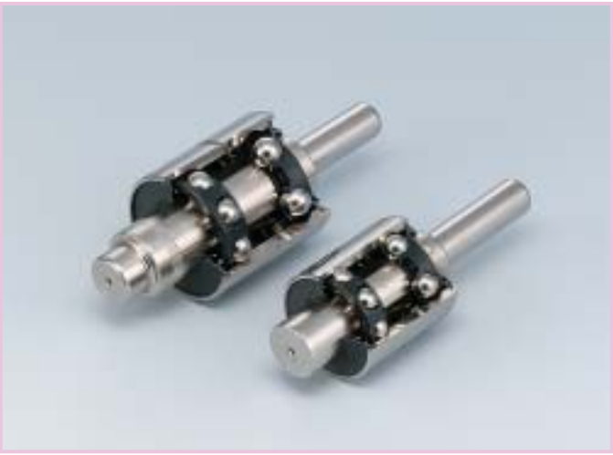
BWFH Type Water Pump Bearings High capacity and high moment rigidity have been achieved by increasing the limited number of balls in the front row.
