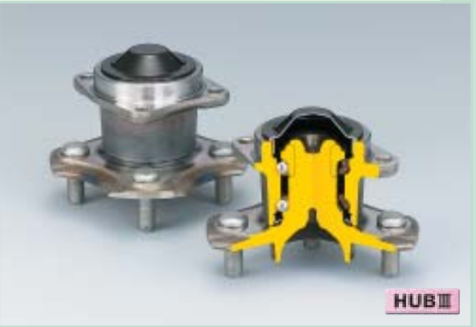
Double-Row Angular Contact Ball Bearings with Inner and Outer Mounting Flange(HUB III for Non-Driven Wheels) Double-row angular contact ball bearing with integral inner and outer mounting flange. Easy incorporation of ABS sensor.
