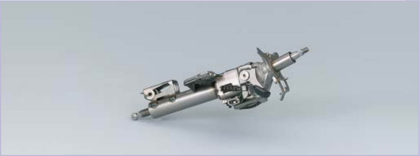
Upper Pivot Tilt Steering Column Tilt steering column with a pivot center in the upper part of the column. Steering wheel position can be adjusted up and down. The automatic tilt-away steering column feature raises the steering wheel for ease when exiting the vehicle.
