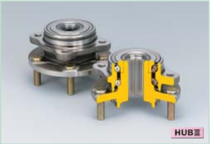
Double-Row Angular Contact Ball Bearings with Inner and Outer Mounting Flange(HUB III for Driven Wheels) Double-row angular contact ball bearing with integral inner and outer mounting flange. Easier mounting because of preset preload.
