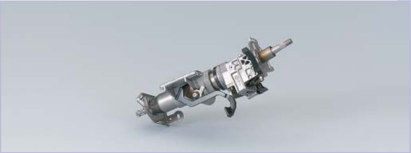
Upper Pivot Tilt and Telescopic Steering Column Tilt and telescopic steering column with a pivot center in the upper part of the column. Steering wheel position can be adjusted back and forth, and up and down. The automatic tilt-away steering column feature raises the steering wheel for ease when exiting the vehicle.
