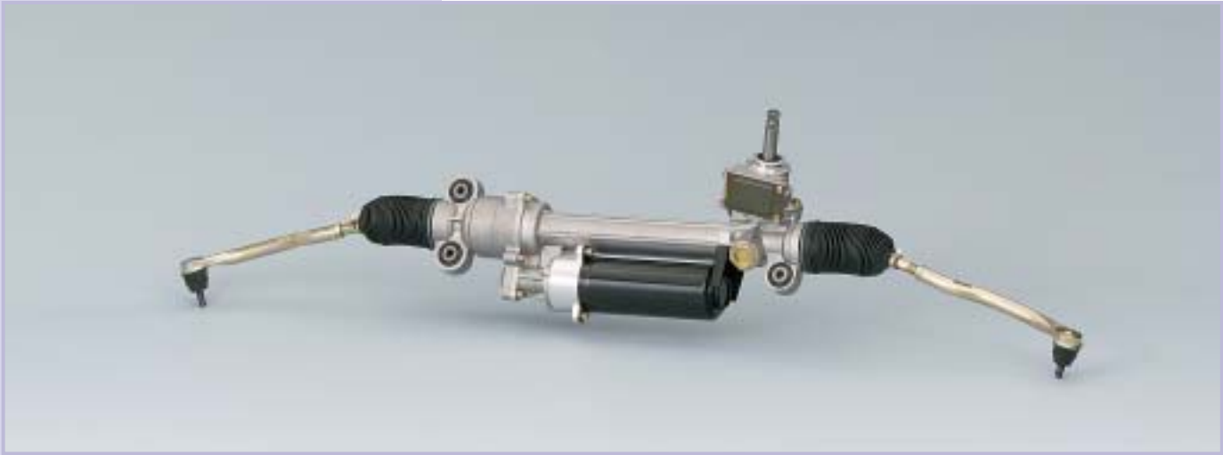
Offset Ball Screw Type Electric Power Steering Offset ball screw type EPS that transmits robust power assist to the rack gear by a highly efficient reduction gear and ball screw.
