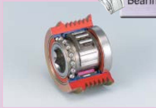
Clutch Pulley Unit for Alternator The pulley unit with a one-way clutch decreases belt noise and extends belt life by absorbing the speed fluctuation transmitted through the crank pulley.
