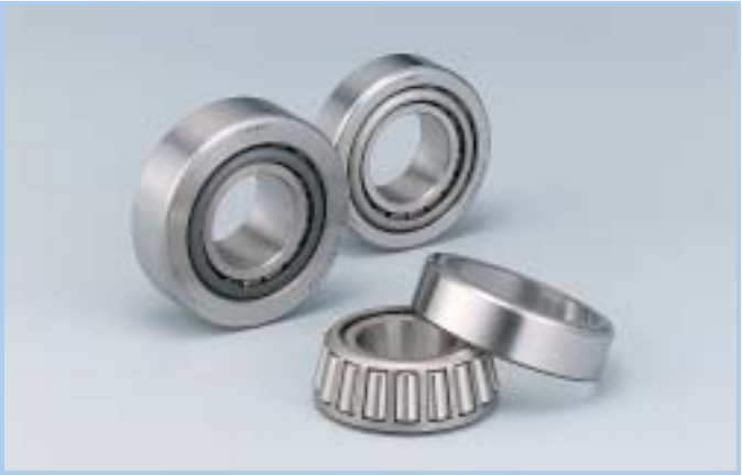
TF(Tough)Series Tapered Roller Bearings Long life in contaminated oil including metal wear powder has been achieved by original materials and heat treatment. Size reductions from standard open type bearings are available.
