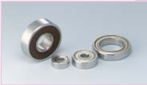
Bearings for Throttle Motor, Bearings for EGR Motor Low torque for low temperatures, and long life under high temperatures have been achieved with newly developed exclusive grease.
