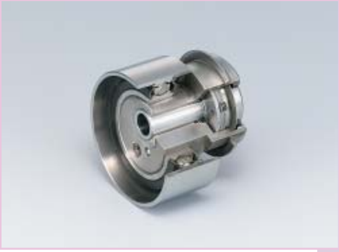
Auto-Tensioner for Timing Belt Optimum timing belt tension has been achieved with a multi-disc damper adjusted to various engine specifications.
