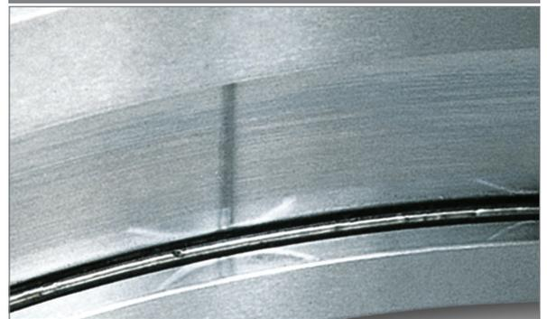
**Possible Causes:** inadequate lubrication, vibration, improper storage
