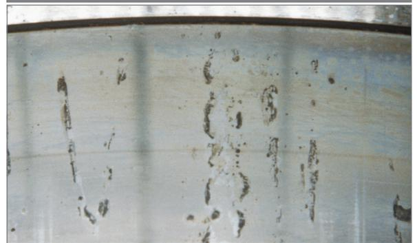
**Possible Causes:** moisture, poor storage conditions, improper handling
