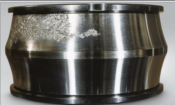
**Possible Causes:** contamination, misalignment, overload, poor lubrication
