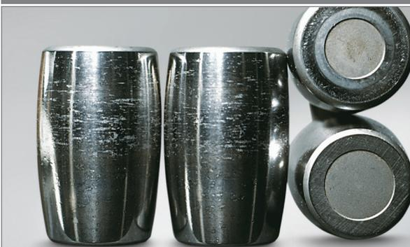
**Possible Causes:** contamination, inadequate lubrication, excessive/improper loading
