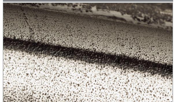
**Possible Causes:** contamination, moisture, inadequate lubrication
