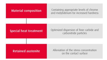
In severe, contaminated, and boundary-lubrication conditions, Super-TF bearings deliver exponentially longer life when compared to conventional carburized bearings. Resulting rate of wear is 1/3 that of standard bearing steel, with 40% greater seizure resistance.
