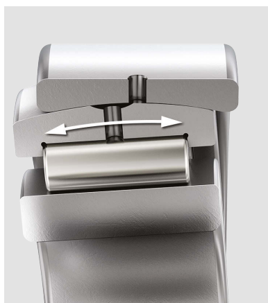
Aligning ring tolerates misalignment and shaft deflection
