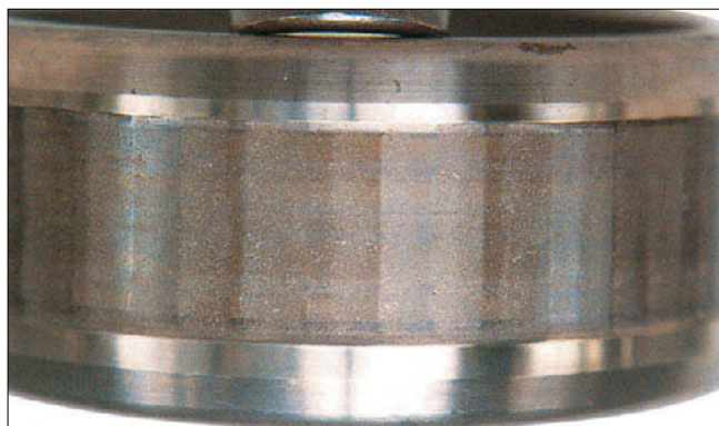
Part: Inner ring of a cylindrical roller bearing Symptom: Many pits occurs due to electrical corrosion; wave-shaped wear on raceway surface Cause: Electrical corrosion
