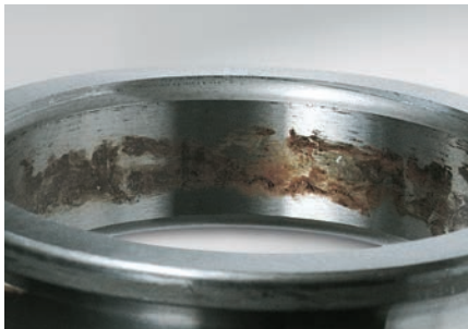
Part: Inner ring of a deep groove ball bearing Observation: Fretting occurs on the bore surface Cause: Vibration
