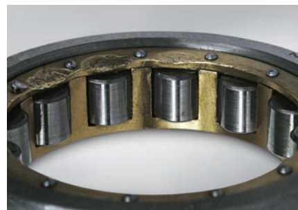
Part: Cage of a cylindrical roller bearing Observation: Deformation of the side face of a machined high-tension brass cage Cause: Large shock during mounting
