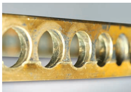
Part: Cage of an angular contact ball bearing Observation: Stepped wear on the outside surface and pocket surface of a machined high-tension brass cage
