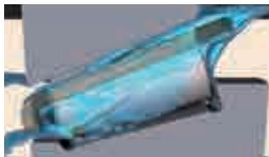
Computational fluid dynamics (CFD) analysis of tapered roller bearings
