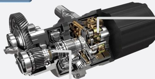
Traction Reducer + Ultrahigh speed motor.
