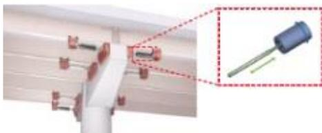
Changes the axial motion caused by earthquake into rotational motion by ball screw
