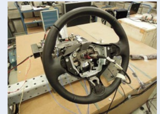
(b) Microphone at the steering wheel center (No. 7)
