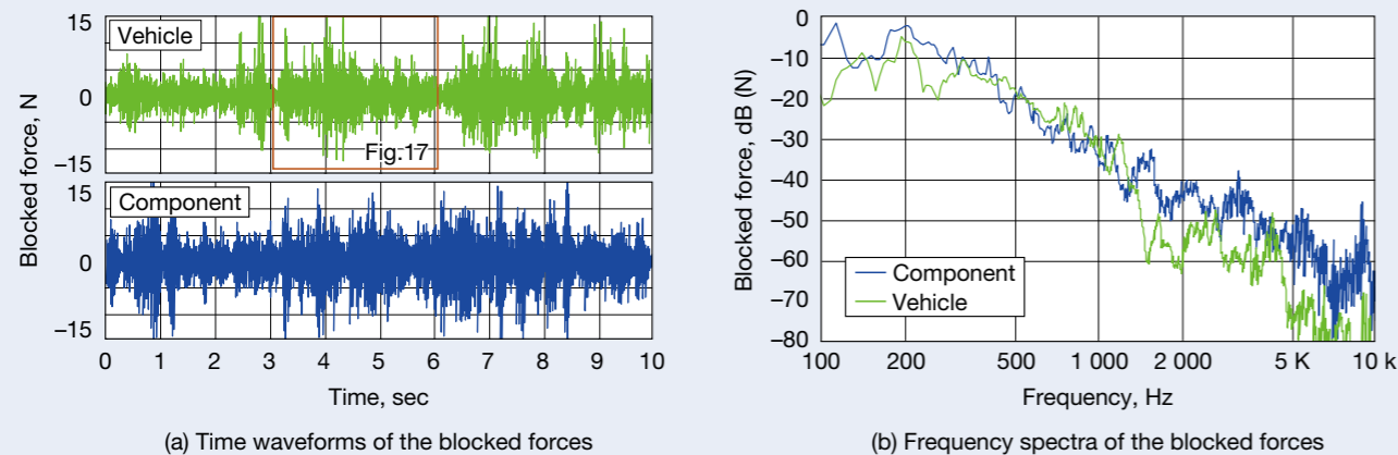
Fig. 28 Blocked forces at the connection of EPS near the accelerometer No. 6 in the X direction. One is identified by inverse matrix method with the regularization factor \phi = 0.03 and vibrations measured by vehicle running test (same with Fig. 17). The other is similarly identified with the factor \phi = 0.001 and vibrations measured by component test.
