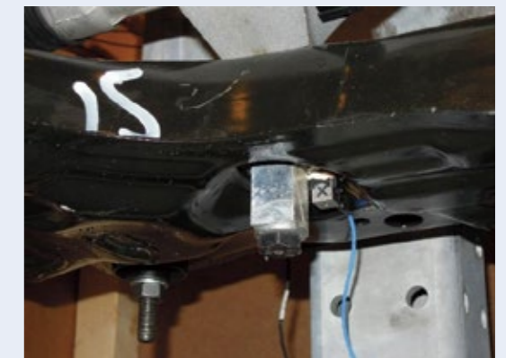
(d) 3-axis accelerometer on the right hand connection of steering gear housing (No. 2)
