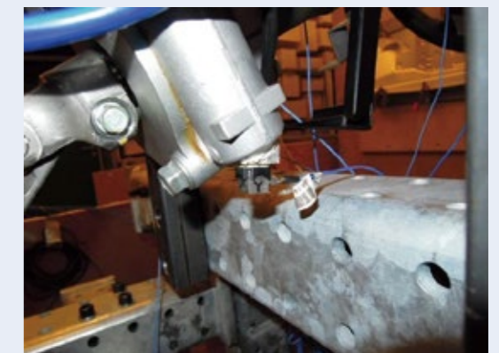
(f) Additional 3-axis accelerometer on the worm/wheel gear housing of steering column (No. 9)
