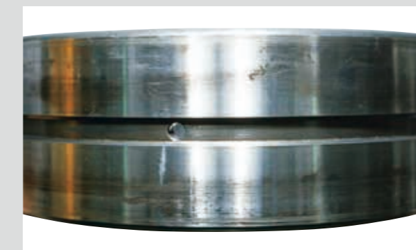
Photo 8 Part: Outer ring of a spherical roller bearing Symptom: Creep over entire circumference of outside surface Cause: Loose fit between outer ring and housing
