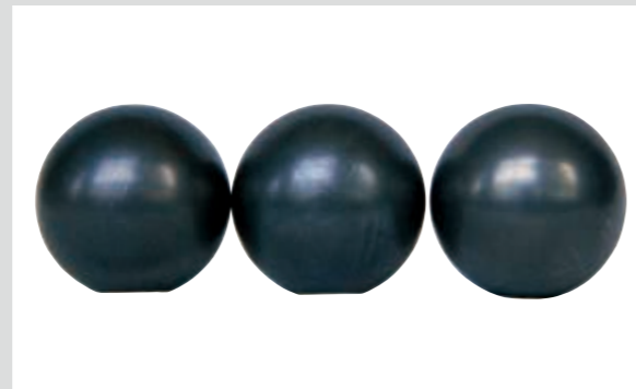
Photo 10 Part: Balls of a deep groove ball bearing Symptom: A dark color covering the entire ball surface
