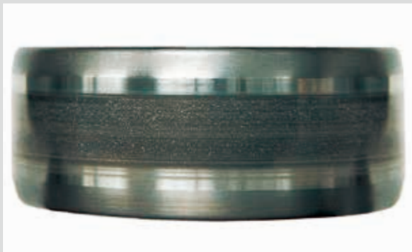
Photo 9 Part: Inner ring of a cylindrical roller bearing Symptom: Belt pattern of electrical erosion accompanied by pits on the raceway surface
