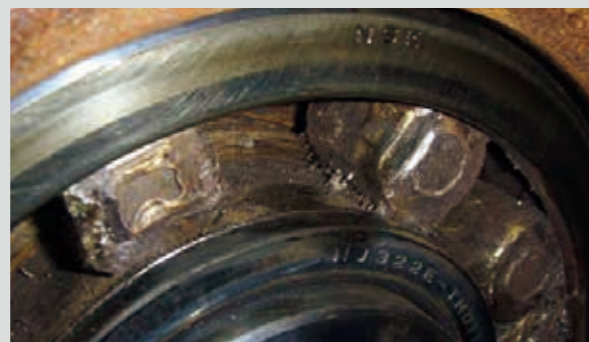
Photo 6 Part: Cylindrical roller bearing Symptom: Seizure of roller at ring raceway surface Cause: Excessively small internal clearance generated heat from motion of the inner ring and rollers under high speed and light load
