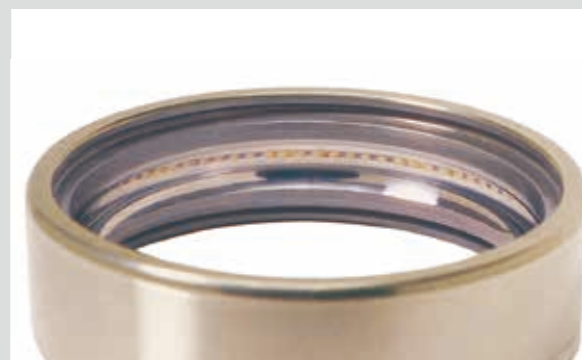
Photo 12 Part: Outer ring of a deep groove ball bearing Symptom: Fluting on the raceway surface (high frequency)
