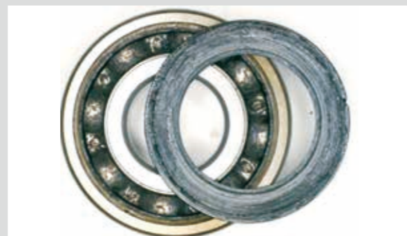
Photo 4 Part: Inside a deep groove ball bearing Symptom: Grease nearly depleted, carbonization Cause: Poor lubrication
