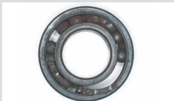
Photo 5 Part: Inside a deep groove ball bearing Symptom: Cage damage, grease nearly depleted, carbonization Cause: Poor lubrication
