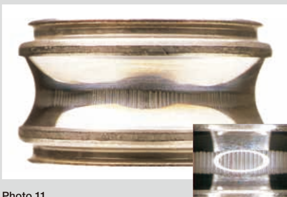
Photo 11 Part: Inner ring of a deep groove ball bearing Symptom: Fluting on the raceway surface (high frequency) Enlargement
