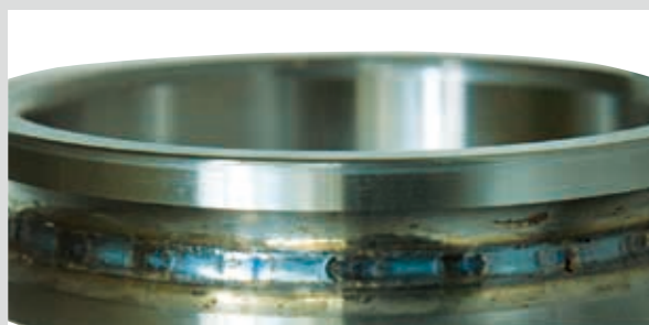
Photo 1 Part: Inner ring of an angular contact ball bearing Symptom: Raceway discoloration, melting at ball pitch intervals Cause: Excessive preload
