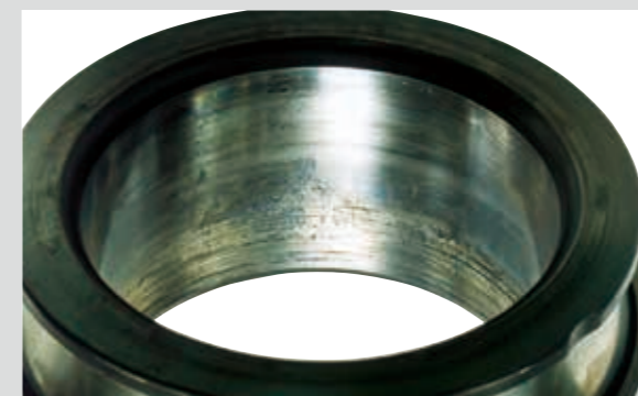
Photo 7 Part: Inner ring of a spherical roller bearing Symptom: Creep accompanied by scoring of bore surface Cause: Insufficient interference
