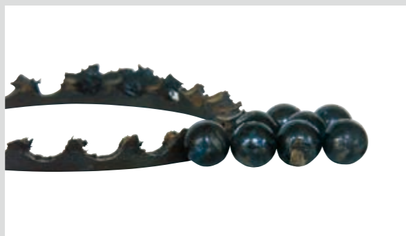
Photo 3 Part: Balls and cage of Photo 1 Symptom: Cage damaged by melting, balls discolored and melted Cause: Excessive preload
