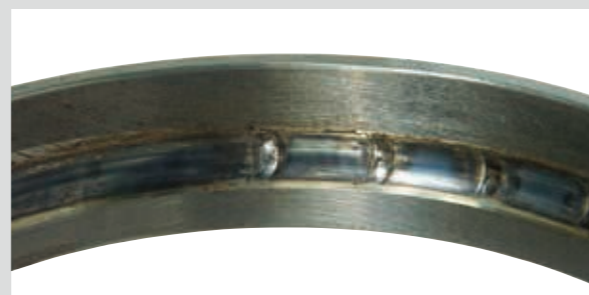
Photo 2 Part: Outer ring in Photo 1 Symptom: Raceway discoloration, melting at ball pitch intervals Cause: Excessive preload
