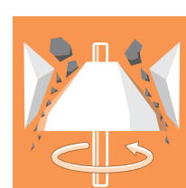
Cone Crusher Material is fed into the crusher cavity and processed by the eccentric rotating action of the inner cone against the outer cone. Work can be reduced to a diameter ranging from 50 mm to 100 mm.
