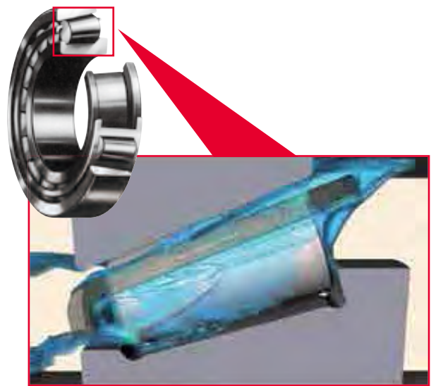
Oil flow analysis of a tapered roller bearing
