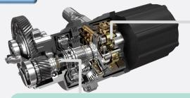
Traction Reducer + Ultrahigh speed motor. Compact, light-weight, Noise reduction
