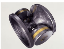
Half-toroidal CVT (continuously variable transmission)
