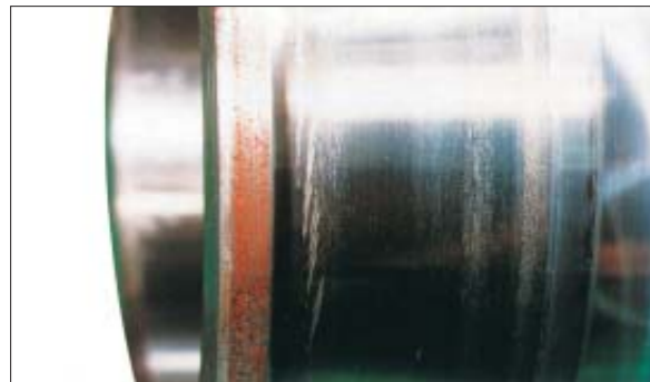
Part: Inner ring of a spherical roller bearing Symptom: Partial smearing occurs circumferentially on raceway surface Cause: Incorrect lubrication
