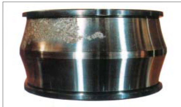
Part: Inner ring of a spherical roller bearing Symptom: Flaking of only one row of raceway Cause: Incorrect lubrication
