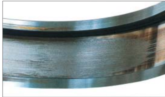
Part: Outer ring of a cylindrical roller bearing Symptom: Smearing occurs circumferentially on raceway surface Cause: Roller slipping due to excessive grease filling
