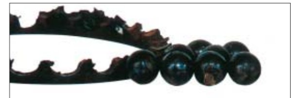
Part: Balls and cage of an angular contact ball bearing Symptom: Cage is damaged by melting; balls become discolored and melted Cause: Excessive preload
