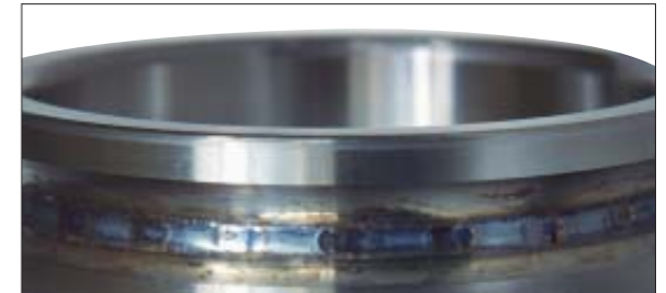
Part: Inner ring of an angular contact ball bearing Symptom: Raceway discoloration; melting occurs at ball pitch intervals Cause: Excessive preload
