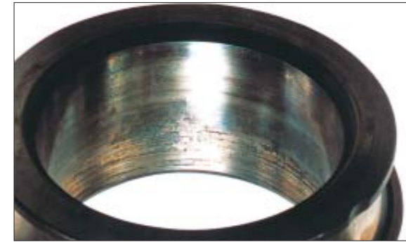
Part: Inner ring of a spherical roller bearing Symptom: Creep accompanied by scoring of bore surface Cause: Insufficient interference
