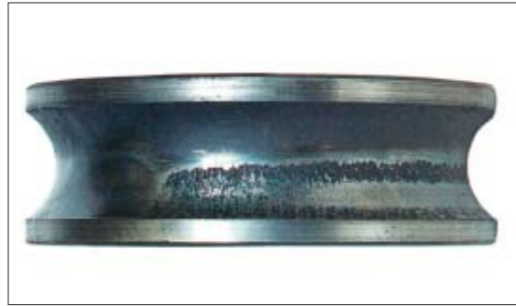
Part: Inner ring of an angular contact ball bearing Symptom: Flaking occurs diagonally along raceway Cause: Improper alignment between shaft and housing during mounting
