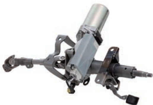
The mechatronic EPS system that combines a motor and the ECU into a single unit
