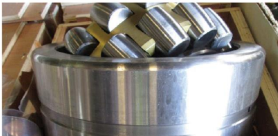
Is it counterfeit? Yes. Things to look for: no lifting holes, corner radius should not be polished, no indent in rollers.
