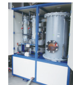
The waste liquid distillation concentrator deployed to Amatsuji Steel Ball Mfg. Co., Ltd. (Shiga plant)
