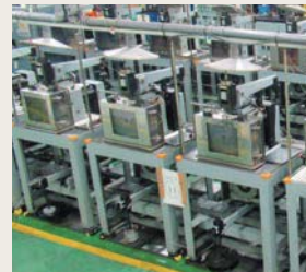
Durability testing machines
