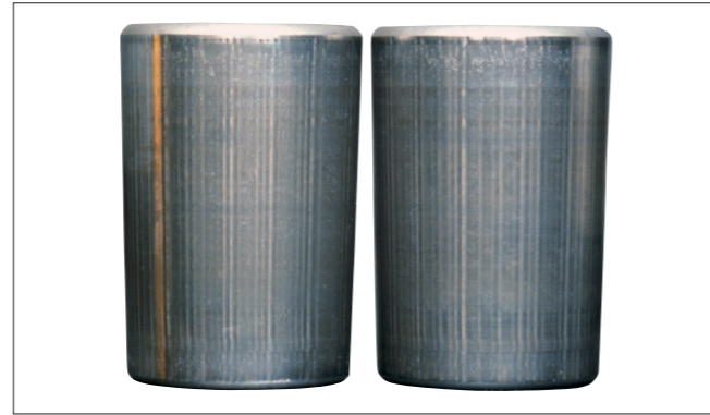
Photo 7-15-2 Part: Tapered rollers in Photo 7-15-1 Symptom: Striped pattern of corrosion occurs on the rolling surface
