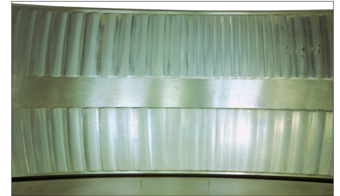
Photo 7-10-2 Part: Outer ring of a spherical roller bearing Symptom: Wear having a wavy or concave-and-convex texture on loaded side of raceway surface Cause: Entry of debris under repeated vibration while stationary
