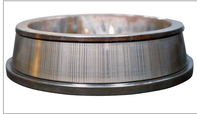
Photo 7-15-1 Part: Inner ring of a tapered roller bearing Symptom: Striped pattern of corrosion occurs on the raceway surface
