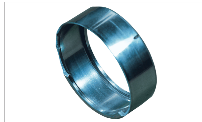
Photo 7-5-4 Part: Outer ring of a solid type needle roller bearing Symptom: Fracture occurs at the outer ring rib Cause: Roller inclination due to excessive loading (Needle rollers are long compared to their diameter. Under excessive or uneven loading, rollers become inclined and push against the ribs.)
