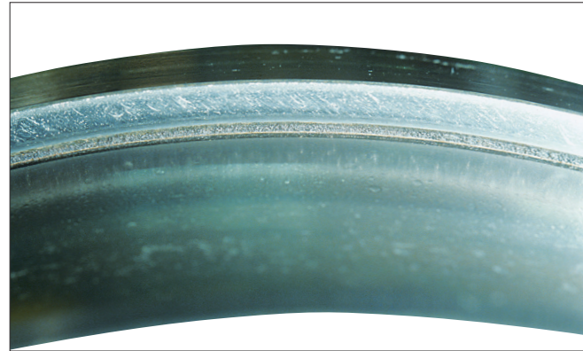
Photo 7-3-1 Part: Inner ring of a spherical roller bearing Symptom: Scoring on large rib face of inner ring Cause: Roller slipping due to sudden acceleration and deceleration
