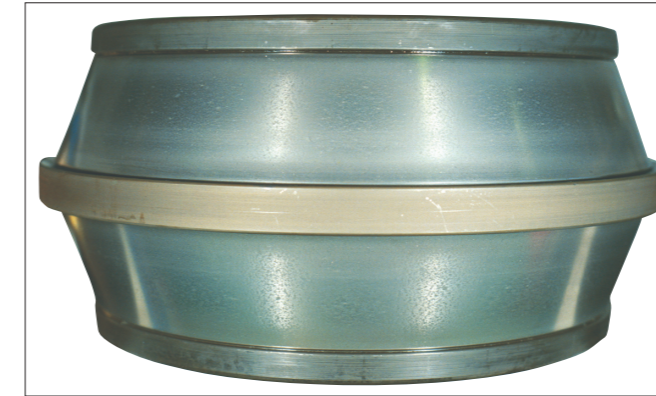
Photo 7-8-1 Part: Inner ring of a double-row tapered roller bearing Symptom: Frosted raceway surface Cause: Debris caught in the surface
