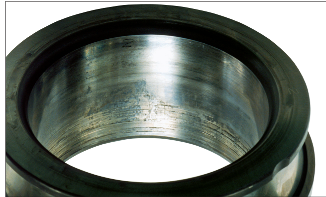
Photo 7-13-1 Part: Inner ring of a spherical roller bearing Symptom: Creep accompanied by scoring of bore surface Cause: Insufficient interference
