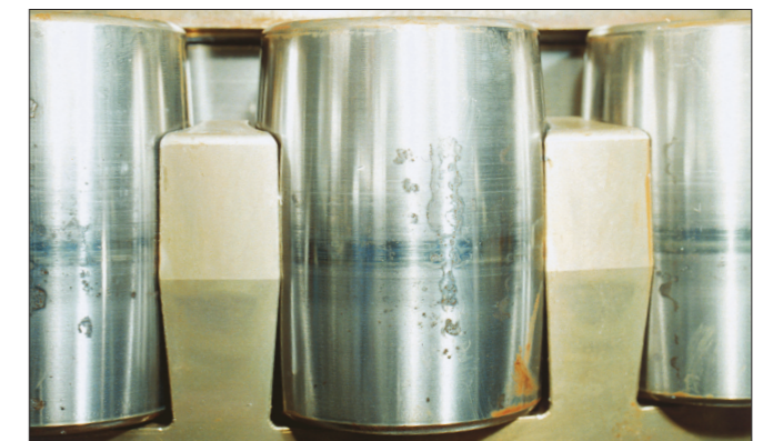
Photo 7-16-4 Part: Rollers of a spherical roller bearing Symptom: Pit-shaped rust on rolling contact surface. Corroded portions. Cause: Moisture condensation during storage
